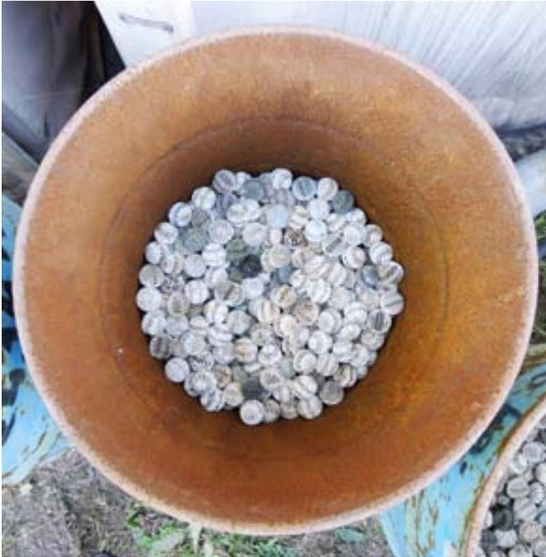
Photo 9 — Barrel of plastic moulded balls used for extracting underground pollutants from contaminated site (Dunaujvaros, Hungary)
